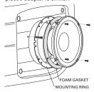
**Figure 4.** Mounting the GTO607C woofer without the metal adapter.
